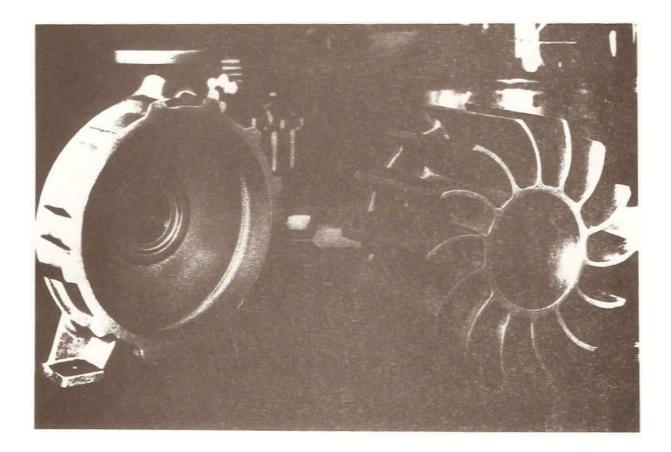
Fig. 19: Pump casing and impeller
