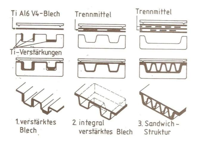
Fig. 26: Superplastic forming and diffusion bonding
