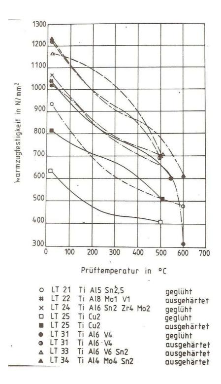
Fig. 14: Warm strength of titanium alloys
