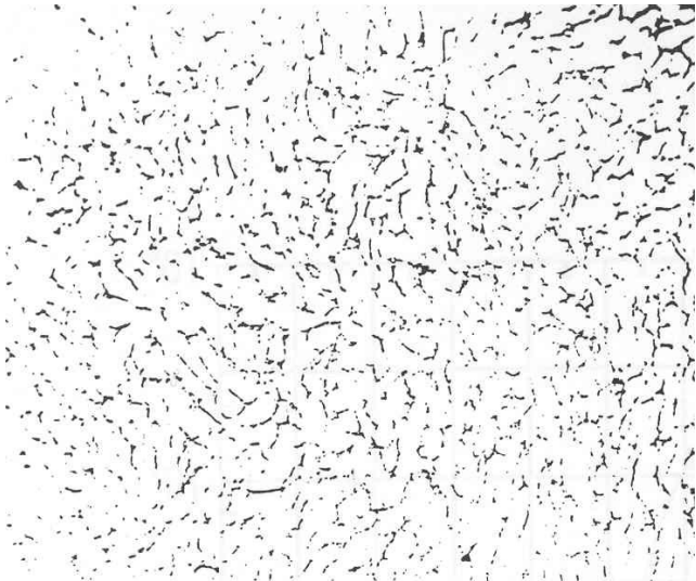
Figure 2 Microstructure in the forged and annealed condition (as delivered state). (x 500)
