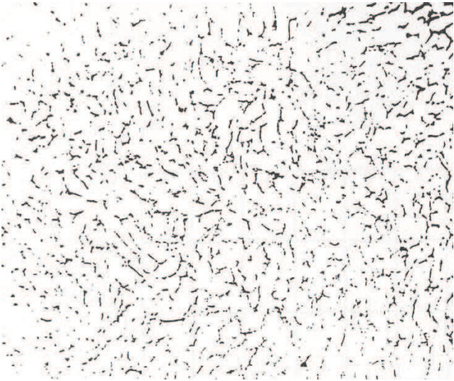
Figure 2 Microstructure in the forged and annealed condition (as delivered state). (x 500)
