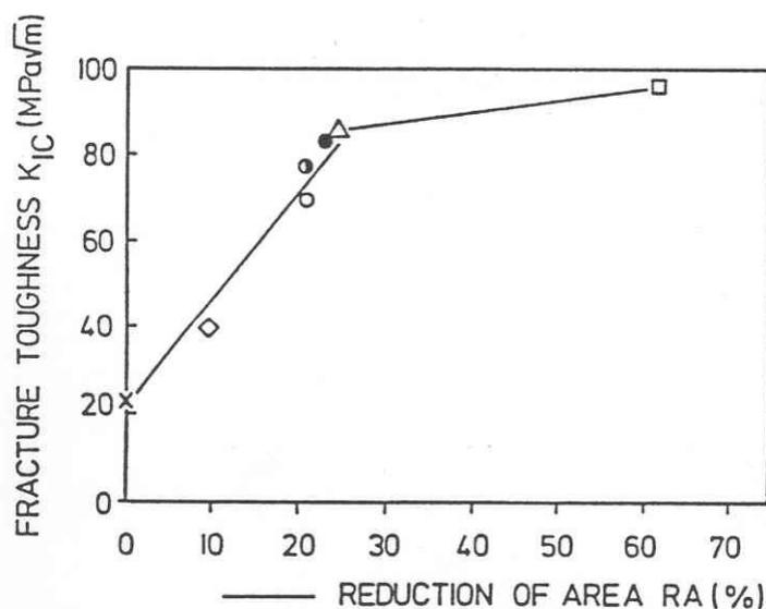
Fig. 11: Relationship between fracture toughness  $K_{Ic}$  and ductility as assessed by reduction of area (RA).
