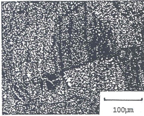
Fig.5: Microstructure after 4 h 440 °C + 16 h at 560 °C
