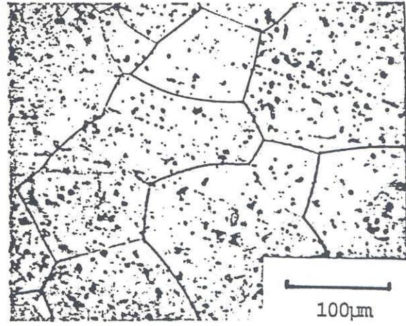
Fig.6: Microstructure after aging 1000 h at 250 °C
